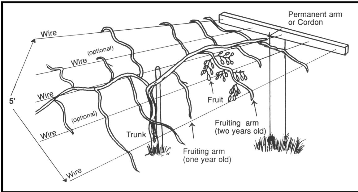
**Figure 1: A Horizontal T-Bar Trellis for Kiwifruit**
